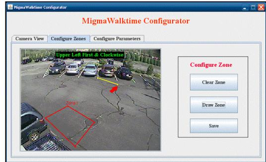
**Step 5:** Touch the lower right corner with the stylus or mouse. This will connect the three points and there will be two yellow lines drawn.
