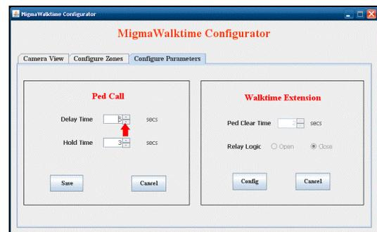
Configuring the **Walktime Extension** is identical to the **Ped Call**. Click on the **Config** button, select your preferred time for Ped Clear Time and your choice for Relay Logic.
