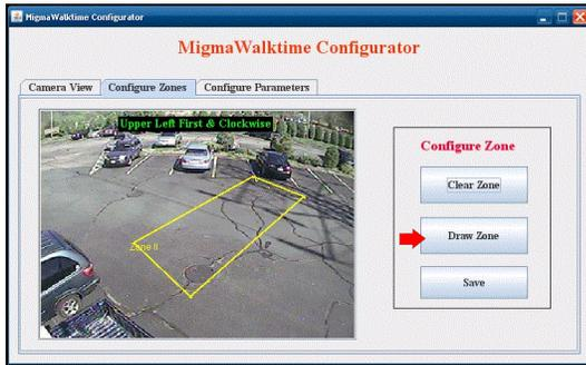
**Step 3:** Now using the stylus or mouse touch the *upper left* corner of the desired zone to start drawing.
