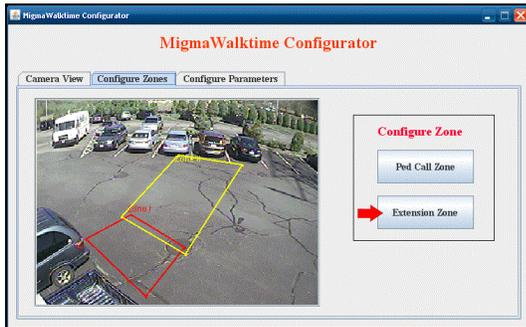
**Step 2:** Click on the **Clear Zone** button to clear the existing zone and then click the **Draw Zone** button. The **Extension Zone** should cover as much of the crosswalk as possible. As long as there are pedestrians detected in this zone, the walk time extension request (i.e., relay contact closure) is sent to the controller until he or she is out of this zone.
