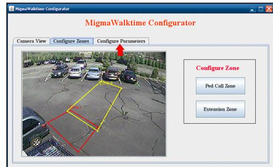
For both **Ped Call**, click on the **Config** button to configure the system for your specific needs.
