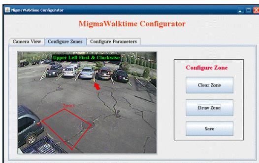
**Step 4:** Now touch the upper right corner with the stylus or mouse. This will connect the two points and there will be one yellow line drawn.
