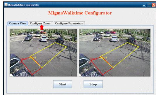
The camera view from System1 is shown. The existing zones are in RED and YELLOW. There are two configuration zones, one for automated ped call, and the other for walk time extension.
