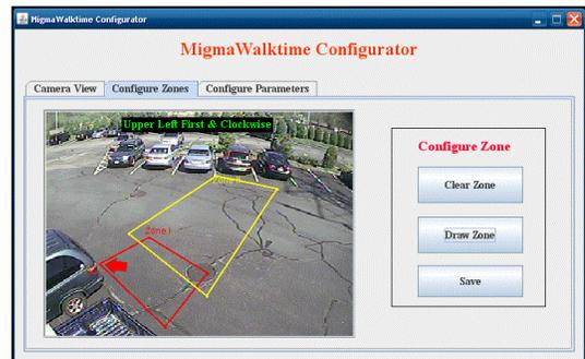
**Step 7:** After completing the zone configuration, click on the **Save** button. This will save the newly configured **Ped Call Zone** to the computer. This is the zone that will be used to detect pedestrians and place a ped call.
