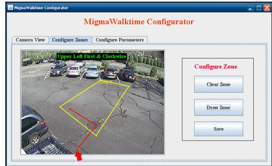
**Step 6:** Finally touch the lower left corner with the stylus or mouse and this will complete the zone by connecting all four points.
