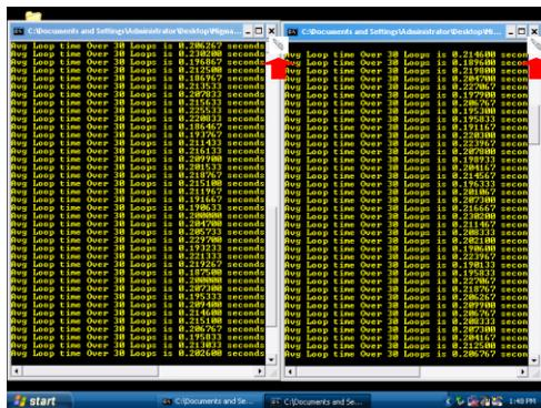
Once connecting to SBC using one of these methods, close both programs (two screens with yellow prints) by clicking on the exit button (X) on top of each DOS window.
