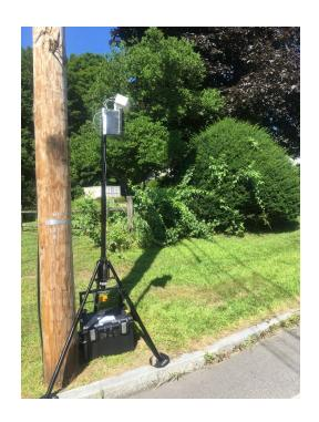
MigmaCount<sup>TM</sup> Mobile is a portable automated passive pedestrian and cyclist counting system. It separates and counts pedestrians and cyclists traveling both individually and in groups. It tracks them through a combination of a high resolution IR LED stereo camera and a high resolution LiDAR. By combining these two sensors, it is capable of counting large or small numbers of pedestrians and cyclists traveling in two directions simultaneously. Major features include:
